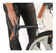
To make the bike more compact, 1) open the seat post quick release and push the seat post into the frame, 2) fold the handle bar grips and pedals.
