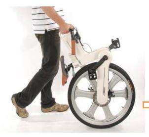
The handle on top of the front fork can be used as a hand hold to roll the bike along during transport.
