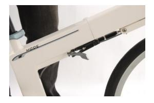
Press pedals outer body inward toward frame and rotate body upward to fold compact.
