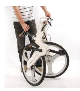
Rock the frame upward with your right hand and pull the front backward and together in one motion so the wheels meet and the magnet catches.
