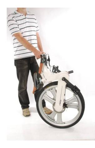
To unfold the IF Mode: unfold the pedals and set left side crank down first, raise the seat and clamp, assemble the left and right handle grip in position.
